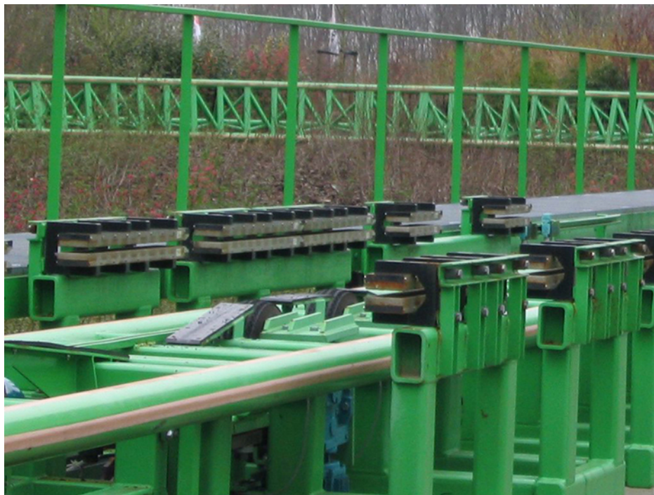
Figure 13.26 The rows of rare-earth magnets (protruding horizontally) are used for magnetic braking in roller coasters. (credit: Stefan Scheer)
